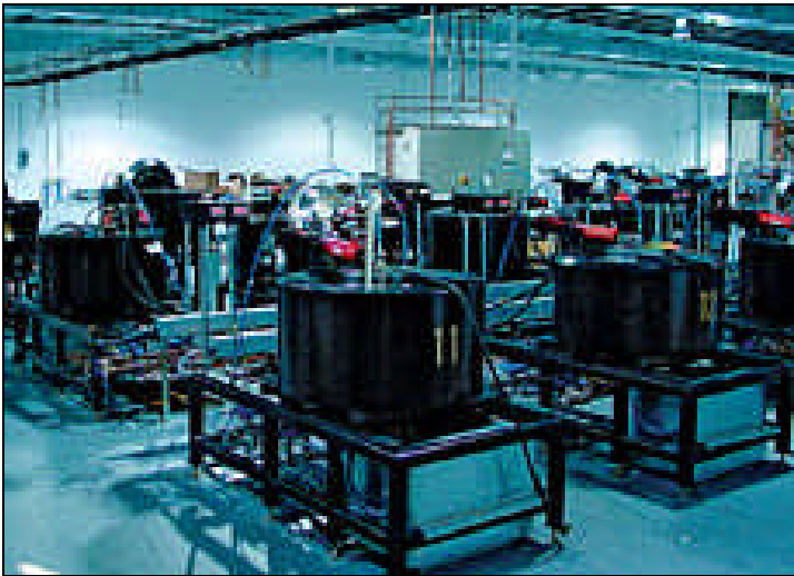
IN THE ROUGH To grow its gem-quality yellow diamonds (a rough one is shown above), Gemesis uses washing-machine-sized crystal-growing chambers to reproduce the high pressures and high temperatures that nature relies on. GEMESIS PHOTOS
