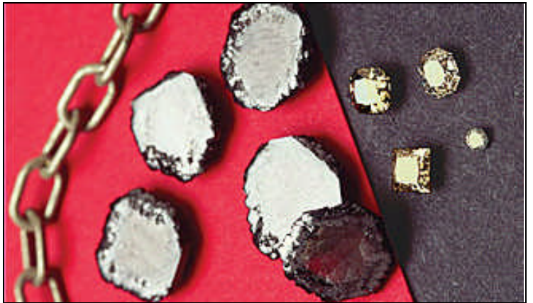
A CUT ABOVE Apollo uses chemical vapor deposition to grow plates of very pure diamond (left) that can be cut and polished into beautiful gems (right). APOLLO DIAMOND PHOTO
