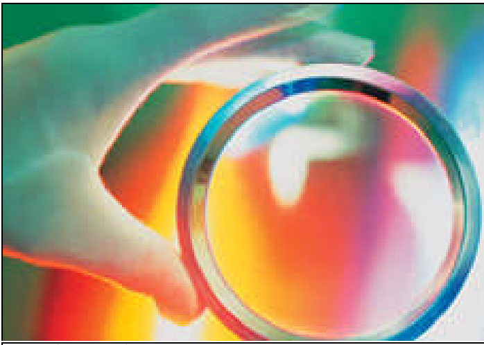
DIAMOND RING Because of its optical transparency, high thermal conductivity, and resistance to chemical attack, synthetic diamond is an attractive material for making optical windows for instruments used in extreme environments.
