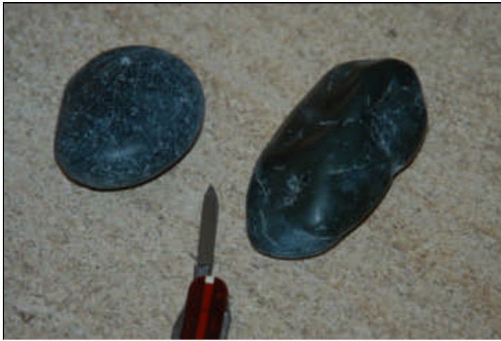
The boulder on the left is serpentine while the one the right of the knife are jade. The knife shown could scratch the serpentine but not the jade.
