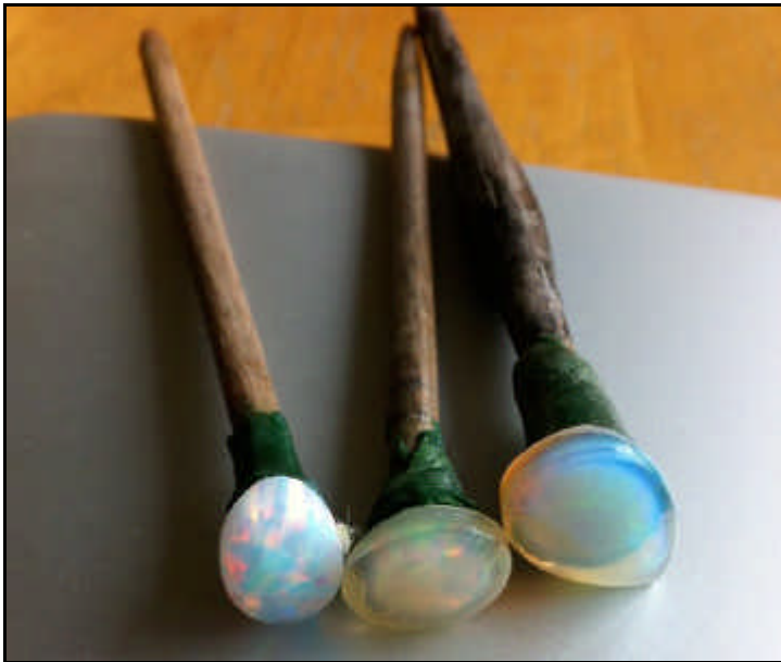
Stones on the dop sticks. Center and right are almost fully "wet". Stone on left didn't make the final stage. All Ethiopian. Stone on right is fine, weeks after finishing..
