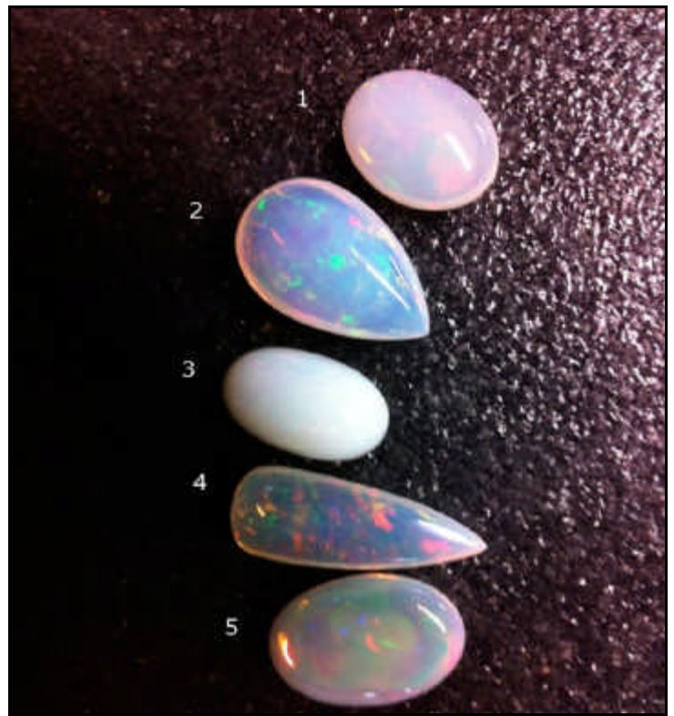
Ethiopian opal in various drying states of the dop. Top to bottom. 1) Still wet. 2) Still wet 3) Really wet 4) Still wet, but drying – see other photo for total transparent stage. 5) wet/dry, not cured fully. Later stones 5, 1, and 3 cracked completely under drying heat (100 watt desk lamp over stoned for 5 to 8 minutes heat test).
