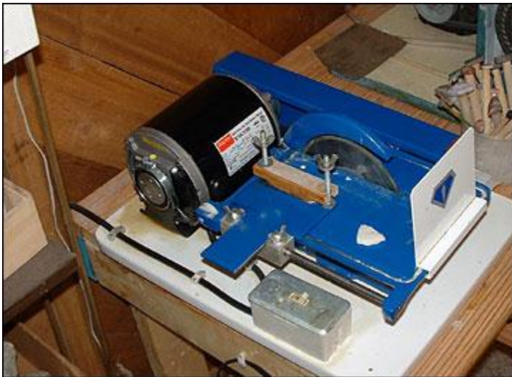
6-inch TC-6 trim saw...careful of the thin blade...it cuts flesh!
