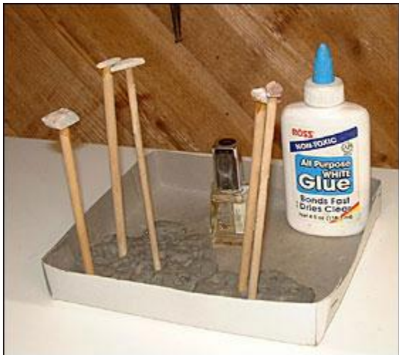
Use wood glue and fingernail polish when thoroughly dry to attach stones to dop sticks.
